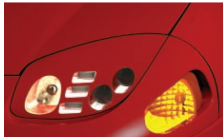
Figure 14: Automotive headlamp modeled in LightTools featuring filament sources for the high beam and LED sources for the low beam.
